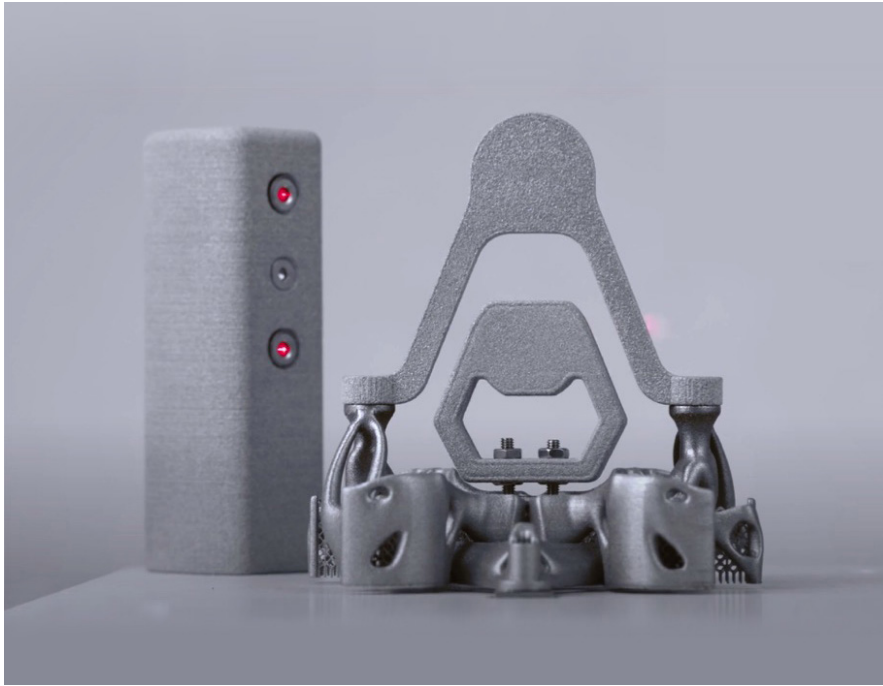
Figure 6 - Compliant mechanisms developed by CSEM in a test configuration.
