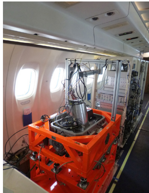
Figure 9 - Quantum gravimeter during an ESA airborne campaign over Iceland.
