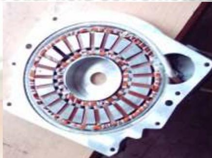
Permanent magnet axial field motors/generators in different configurations
