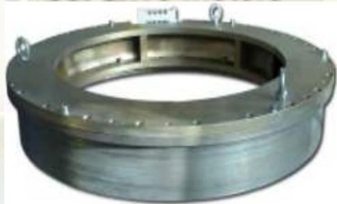
Direct drive motors eliminate the need for gearboxes, worm-gear drives, or other mechanical transmission elements and enable a direct coupling of the payload to the drive. This enables a drive with high dynamic response without hysteresis.
