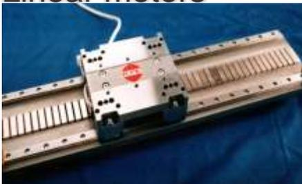
Flat construction with iron core
