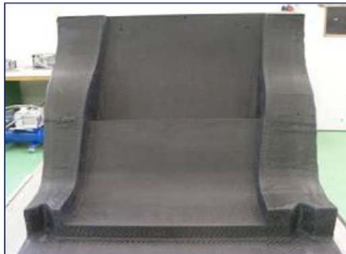
Carbon foam tooling for test panels 1 A/B and 2A, 2B
