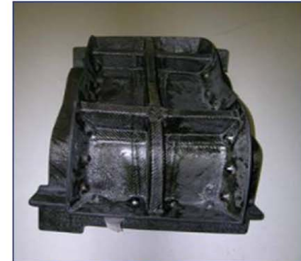
Backside ribbed to improve dimensional stability
