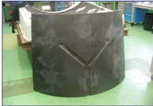
Ceramic foam tooling for parachute door test panel
