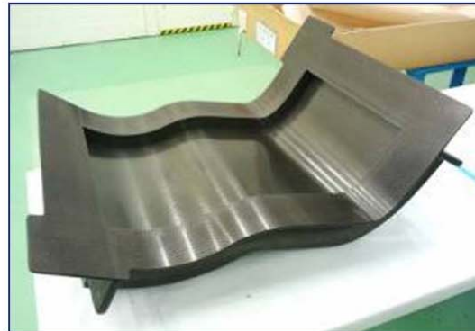
CFRP tooling for test panel 2C
